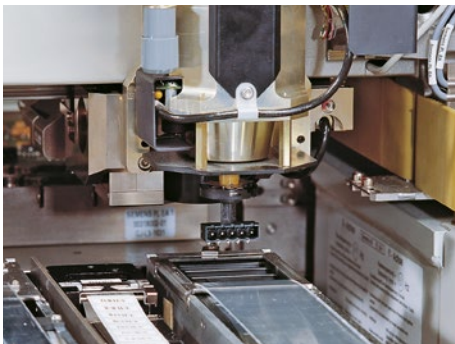
Fig. 49: Component picked from the tape
