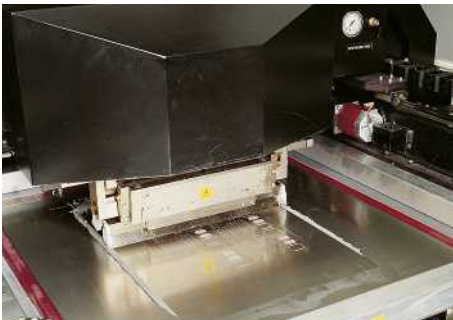
Fig. 40: Squeegee blade system for applying solder paste
