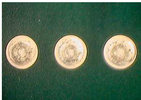
Fig. 71: Assessment of the perimeter wetting and soldering pad wetting not defined in IPC
