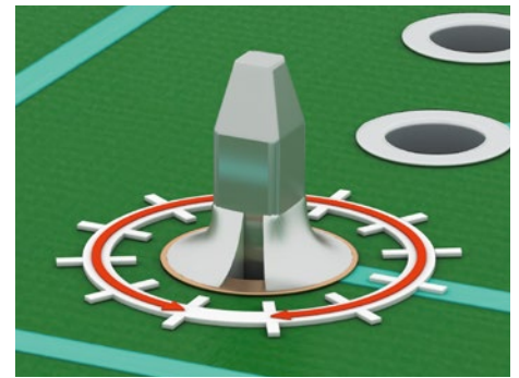
Fig. 64*: Wetting of secondary side 330° or 92%
