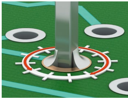
Fig. 63*: Wetting of primary side 270° or 75%
