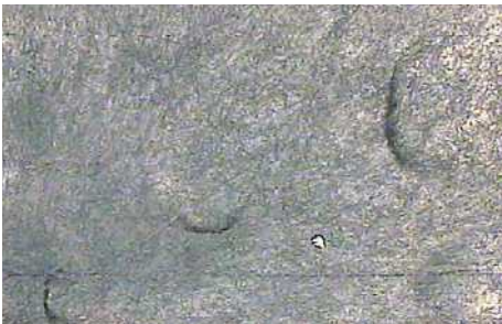
Fig. 29: Failed level – blister formation
