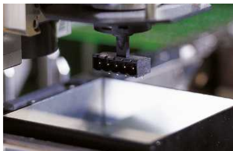
Fig. 50: Camera image capture for component measurement
