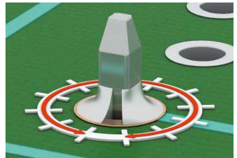
Fig. 64*: Wetting of secondary side 330° or 92%
