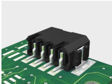
Fig. 11: Example of a recommended layout for an SMD connector
