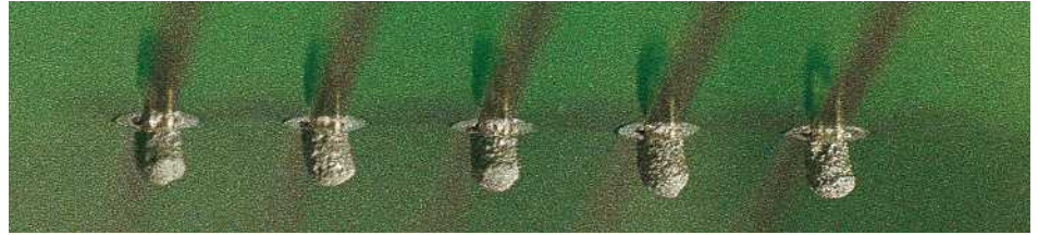
Fig. 58: Paste drops on pin tips
