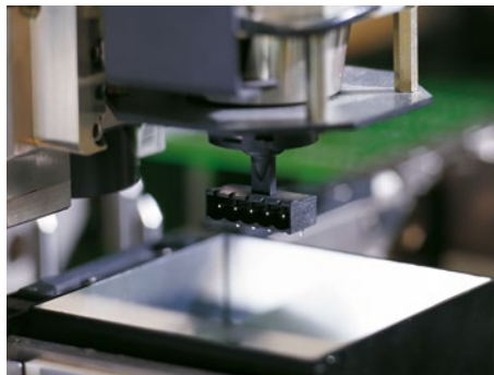
Fig. 50: Camera image capture for component measurement
