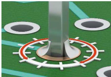
Fig. 63*: Wetting of primary side 270° or 75%
