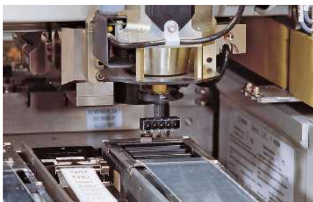
Fig. 49: Component picked from the tape
