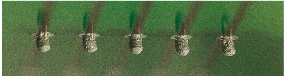
Fig. 58: Paste drops on pin tips
