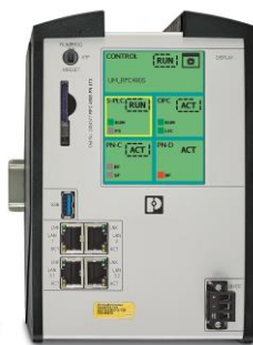
Figure 4 - The resistive touch-capable display is used for programming and diagnostics
