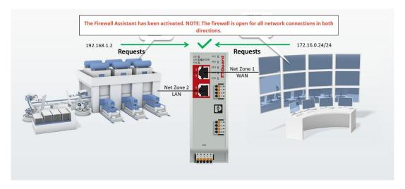
As soon as the start button in the mGuard web-based management is clicked, all incoming and outgoing data traffic is allowed through, and the communication relationships are recorded and prepared accordingly as "Allow rules" in the device. There is no live view of the communications, the users must stop ... the capturing before continuing.
