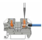
The PTV terminal block family combines the advantages of tool-free Push-in connection with the lateral conductor routing of a screw terminal block. The PTV terminal blocks thus offer direct, fast connection technology and clearly arranged wiring without bending radii in a single terminal block.
