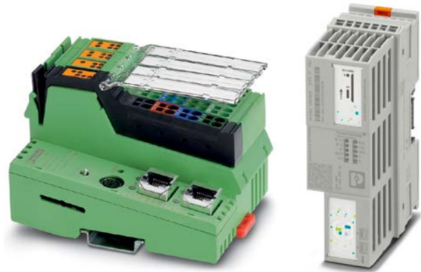
Figure 5: The current IMS operates on Phoenix Contact’s ILC 191 programmable logic controller (PLC), but the next generation will move to the AXC F 1152, a Linux-based controller built on Phoenix Contact’s PLCnext Technology.
