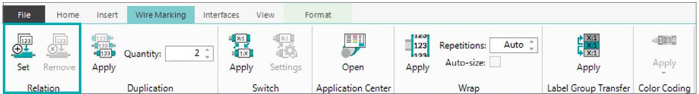
The Set Relation feature allows you to set the relation from the label to the wire to organize individual markers or multiple markers in a file, providing easy organization of markers to wires.
