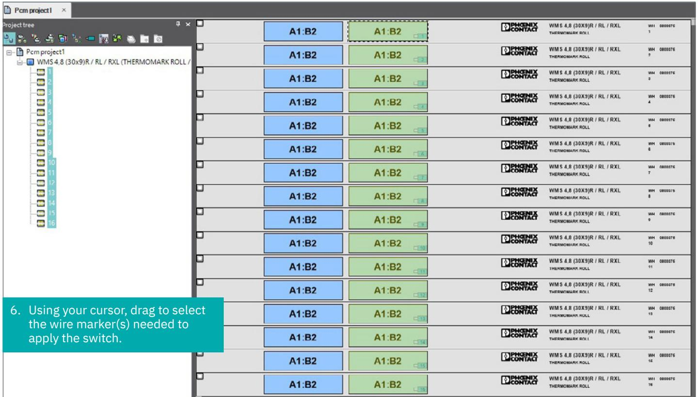
6. Using your cursor, drag to select the wire marker(s) needed to apply the switch.
