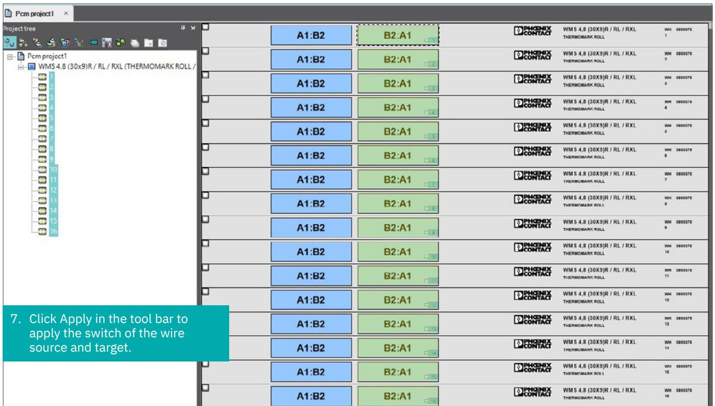
7. Click Apply in the tool bar to apply the switch of the wire source and target.
