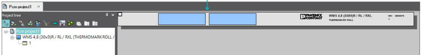
2. Using the text tool, mark the first label with the wire source (A1) and the wire target (B2), separated by a colon
