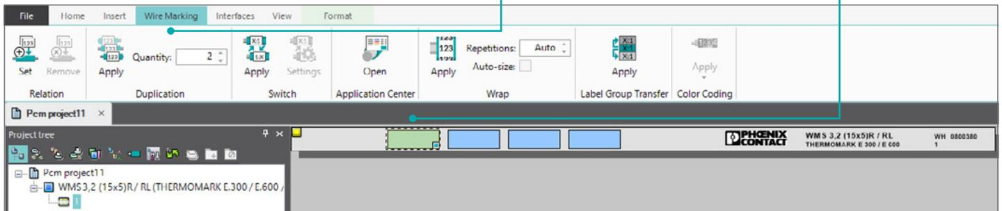
4. Click the Set button located in the Relation section of Wire Marking. This will automatically set the marker relation to wire #1.
