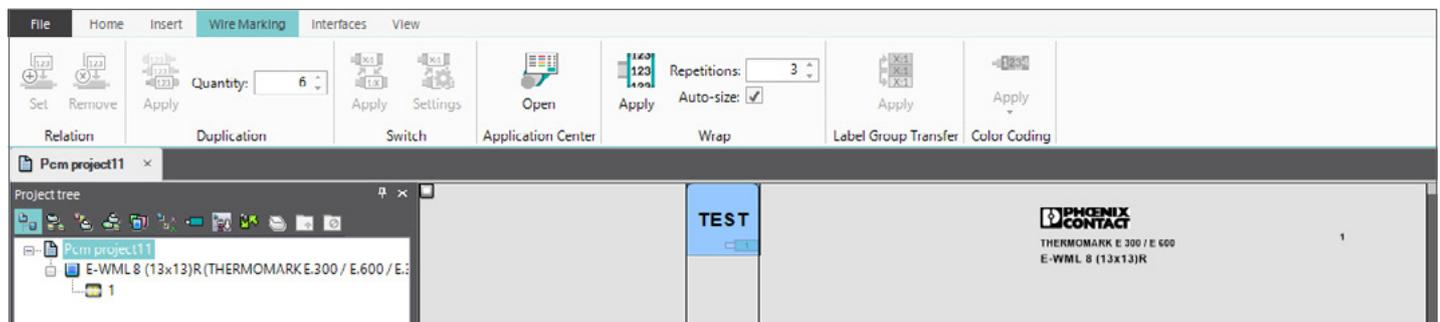
1. Open a blank marker file and add one single line of text to the marking area
