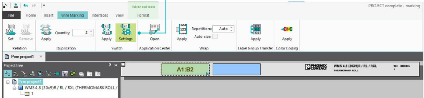
5. In the Switch settings window, specify the switch indicator by highlighting it with your cursor. In this case, it is the colon. The switch indicator can be any other character if the character is specified as the switch indicator. Click Save. Example: A1/B2, A1-B2, etc.
