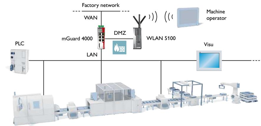
Secure integration of mobile end devices with one-time passwords and DMZ
