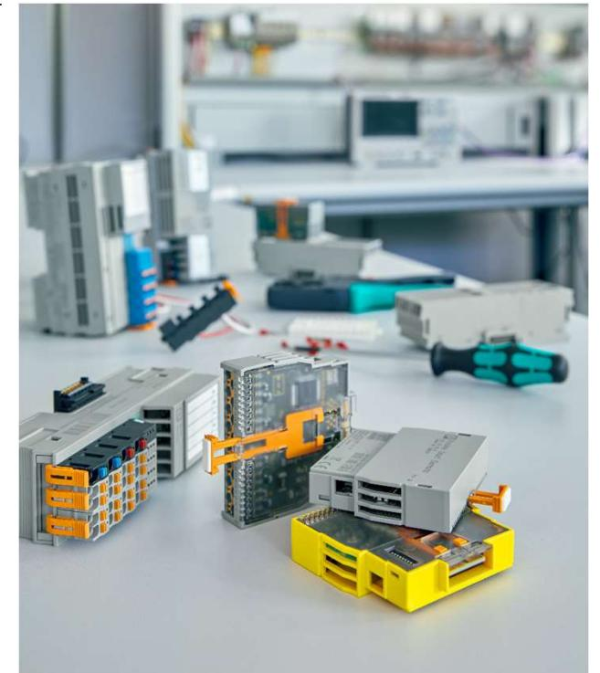
Axioline F - the block-based modular I/O system
