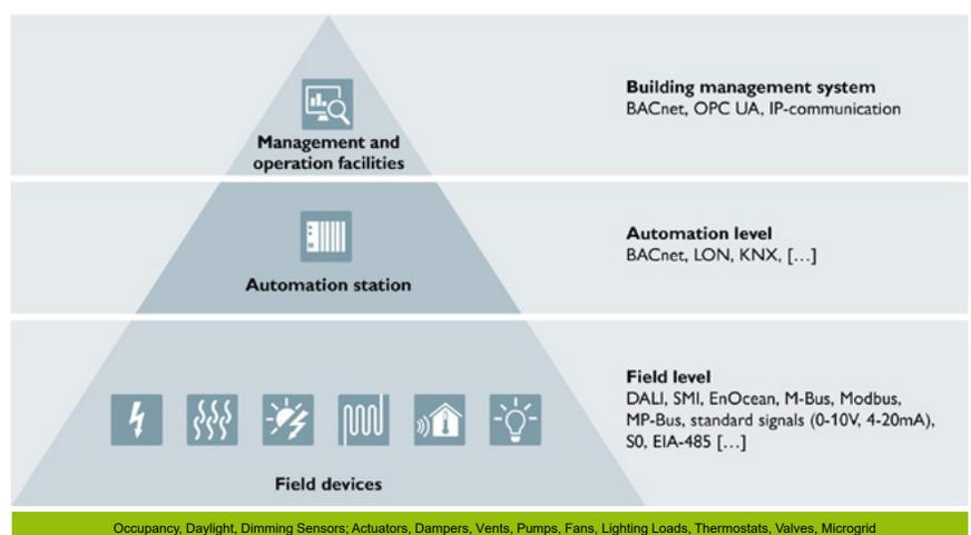
**Figure 1:** Common building automation and control systems
