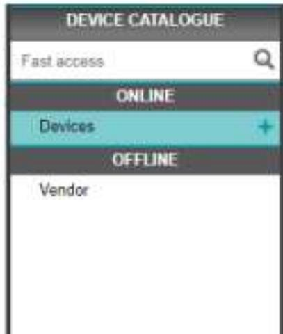
When there is an active TCP/IP connection between IOL-CONF and AXL F stations, the AXL F station along with the connected IO-Link devices can be displayed and parameterized in the ONLINE area (numbering).
