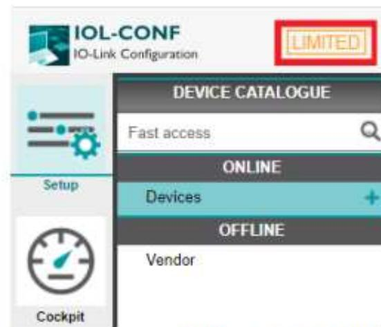
Figure 3-1 “LIMITED” marking in the user interface
