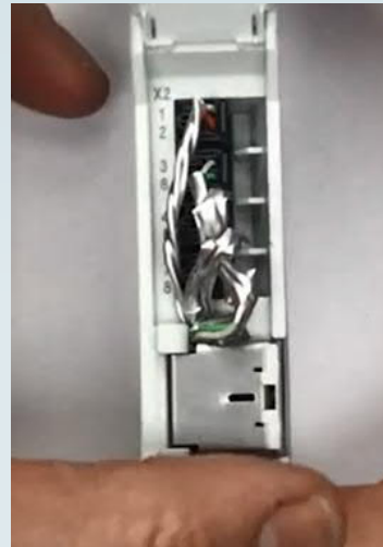
Closing the shield clamp with one finger
