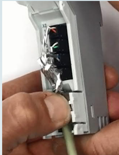
Closing the shield clamp with one finger
