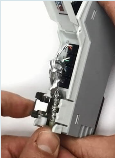
Laying the cable jacket and shielding underneath the shielding clamp
