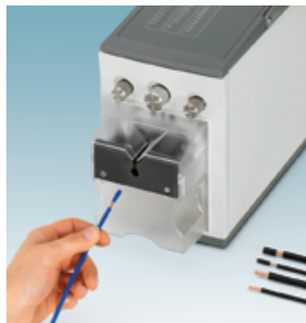
Automatic wire stripping Reference page 60
