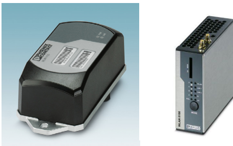
Figure 1A/1B: The FL WLAN 1101 and 5111 both offer high-performance wireless Ethernet, but the different packaging styles make them suitable for different installations. The FL WLAN 1101 has IP housings for easy mounting outside of control cabinets, while the FL WLAN 5111 is designed for easy DIN rail installation.
