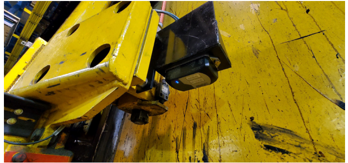
Figure 2: The vertical axis had limited space in the current enclosure, so the FL WLAN 1101's IP housing and flexible mounting options made installation easier.
