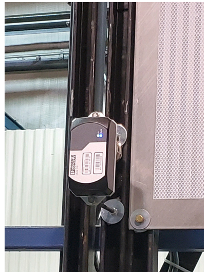
Figure 3A/3B: Although the control cabinet used in the horizontal crane had limited space, the narrow FL WLAN 5111 fit the requirements.
