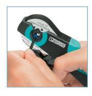
The self-adjusting crimping tools have just one insertion shaft, which adjusts itself automatically to the cross-section to be processed when actuated. Based on this, they are also ideally suited for other conductor standards (JIS/AWG) and for TWIN ferrules. The special mechanism enables square and hexagonal crimp forms.
