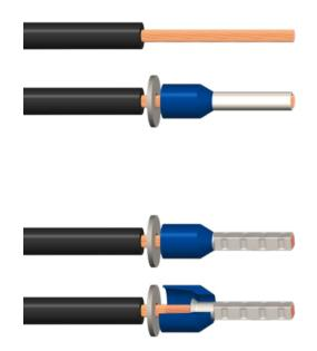
Remove the insulation to a length sufficient to enable you to place a steel washer suitable for the cross-section behind the sleeve. Make sure that no litz wires are damaged or broken
