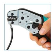
This widely used and universal type of crimping pliers is based on the scissors principle and is available with dies for different types of contact. With these tools, each cross-section has its own die cavity. This means that careful attention must be paid to correct positioning.
