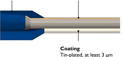
\* Note: In the manufacturing process, the "pulling" action applied to the copper sleeve results in an increase in material hardness. To meet the specifications of DIN 46228, the sleeves must then be annealed. If the material hardness is too high, the crimping process would result in insufficient forming and/or cracks.
