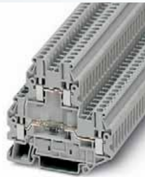
2.5 (4) mm 2 , 28 A，双层接线端子，带 LED
