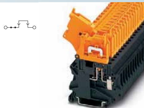
4 (6) mm 2 , 20 A, 悬臂式分断端子, 形状相同, 带测试插座螺钉
