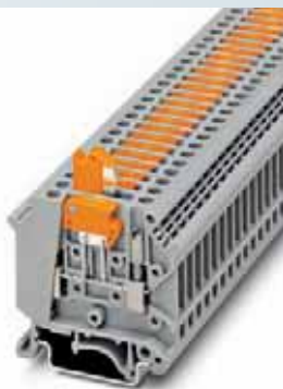
4 (6) mm², 16 A, 刀闸分断端子, 带测试插孔螺钉
