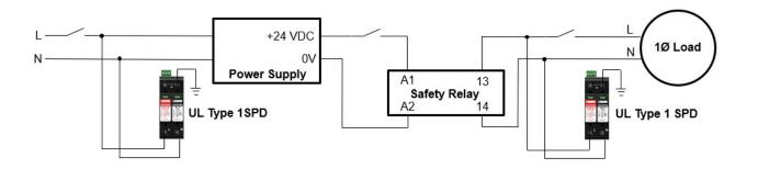
Surge protective devices for the power supply must be installed as close to the power input point as possible. The VAL-US Series makes product selection particularly easy. As UL Listed Type 1 devices, they can be deployed anywhere within the electrical distribution. In addition, the intensity of transient activity within the electrical system may require higher-capacity SPDs.
