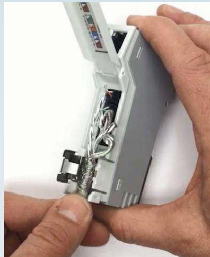
Step 2: Laying the cable jacket and shielding underneath the shielding clamp
