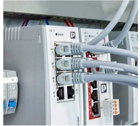
Ideal for building applications due to the LSZH cable sheath
