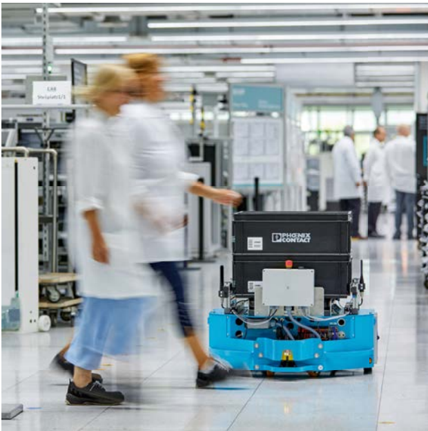
Automated guided vehicle system in production
