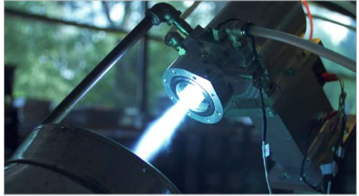
Figure 3: Creating plasma at atmospheric pressure involves temperatures up to 6,000 degrees Celsius.
