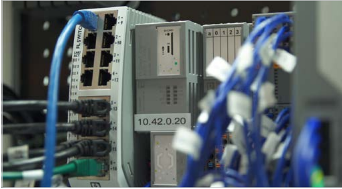
Figure 4: PLCnext Technology offered programming in high-level languages and could communicate with all the required industrial protocols
