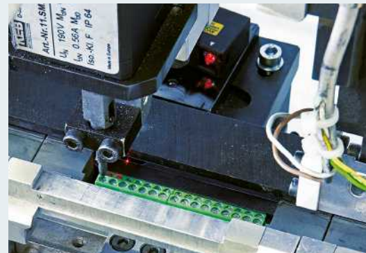
Fully automatic screw test in the manufacturing process
