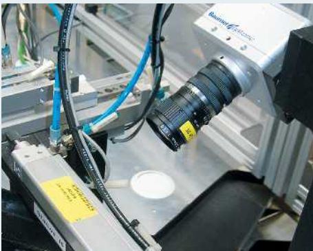
Quality inspection using optical camera systems
