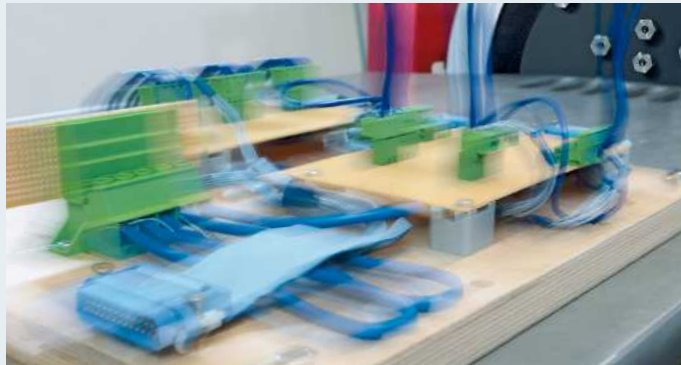
Mechanical load tests through vibration tests
